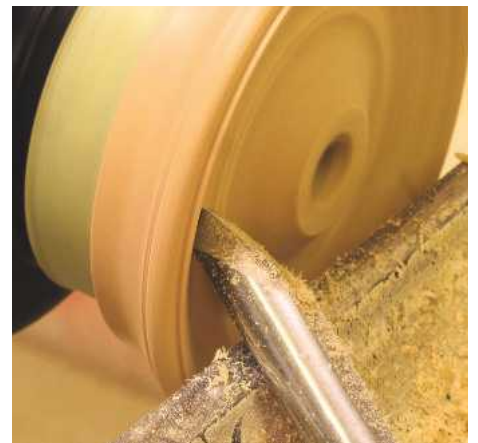
▲ Pic.18 This picture clearly shows the bevel of the tool in contact with the wood. This can only be achieved by dropping the tool handle during the cut
